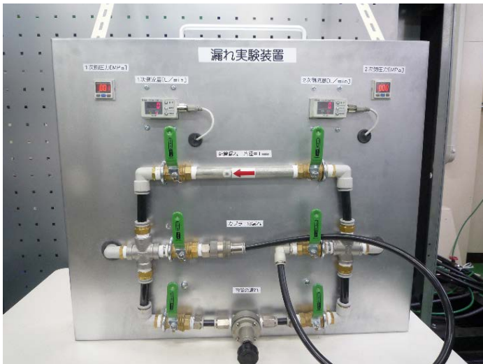
(2) Leakage from a coupler
