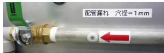
(2) Leakage from a coupler
