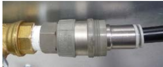
(2) Leakage from a coupler
