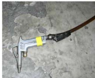
point; air gun 49. 2L/min
