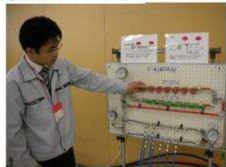
Pressure loss caused by different types of valve
